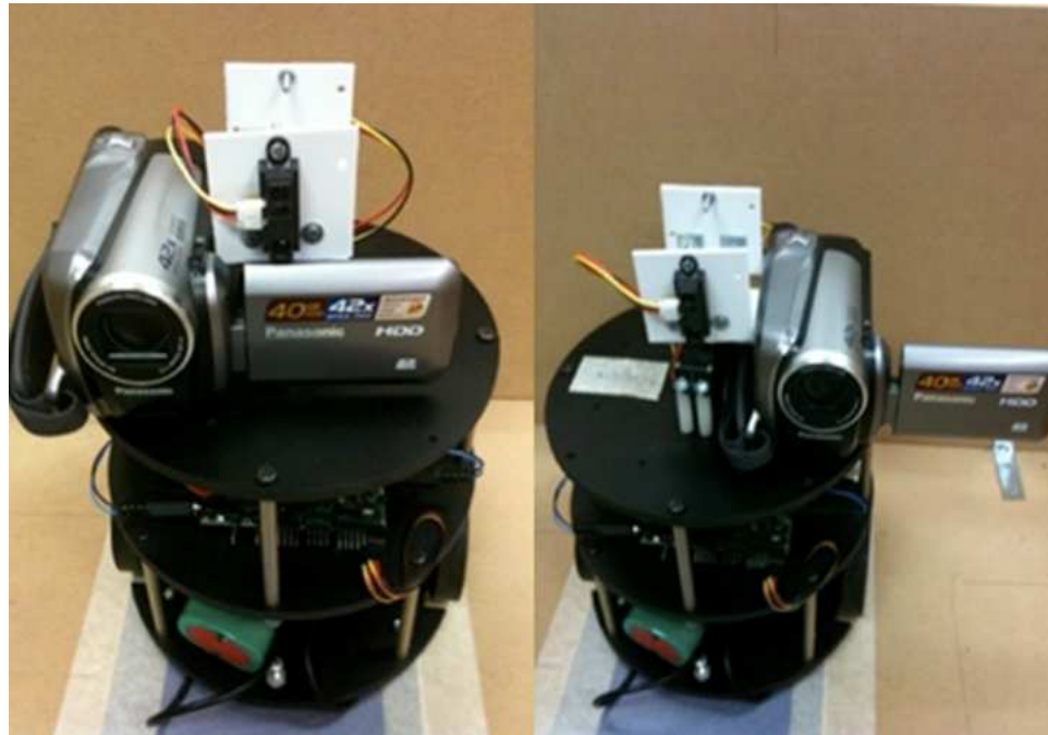
Figure 5.2: Simulating stereo imaging. Right mounted and left mounted on chassis.
