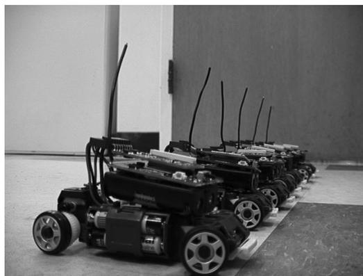
**Figure 1. A line of CotsBots. Over 80 robots have been built to date.**
